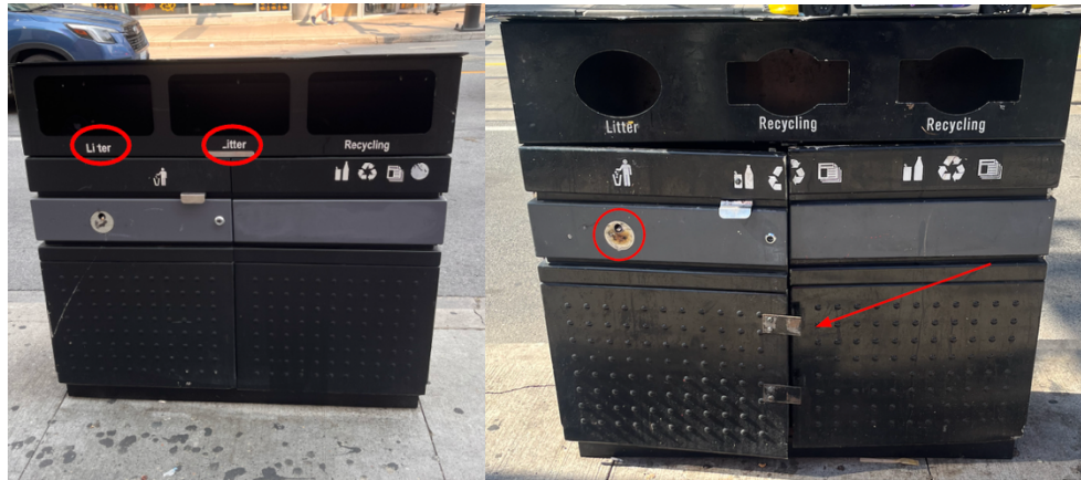
Figure 12. The figure demonstrates the common decal and break-in concerns of the Astral WR4 and WR5 models. Peeling signage/lettering and damaged cigarette receptacles was persistent among them. The WR4 Astral image also shows an example (marked by an arrow) of a bin break-in with the doors left open.
